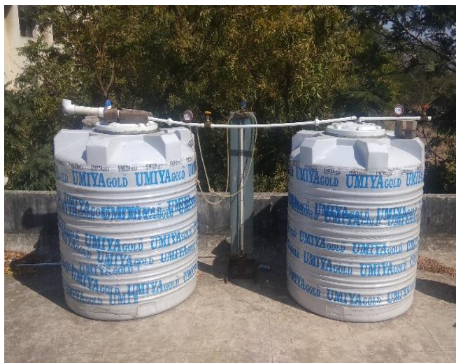
Fig 2. Anaerobic digester set up
